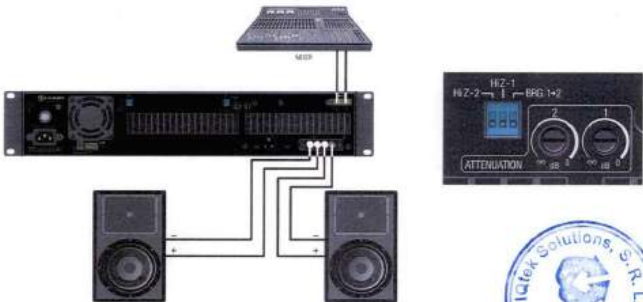
Figure 6 System Wiring Dual Mode
