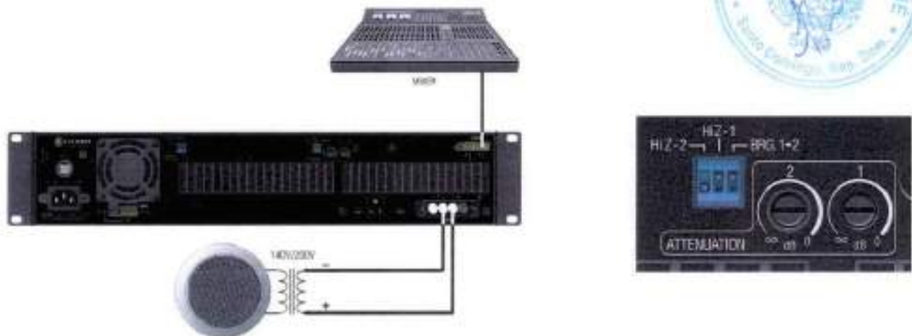
Figure 9 System Wiring for 70V/100V Operation
